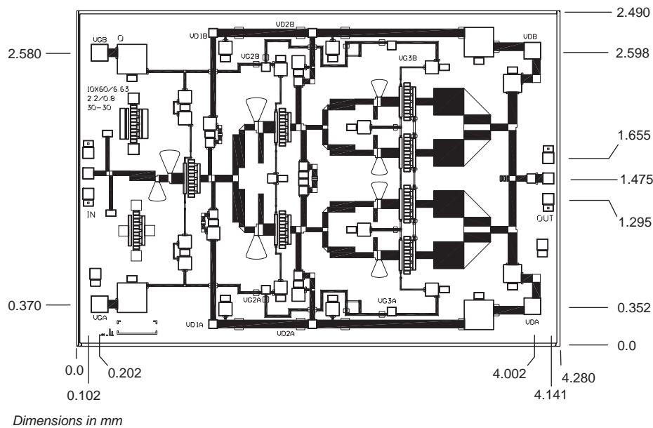
Figure 2. Chip Layout and Bond Pad Locations (Chip Size is 4.28mm x 2.90mm x 50µm. Back of chip is RF and DC Ground)
