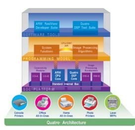
By pairing the ARM CPU core with the Quatro DSP core, the Quatro solution provides OEMs with a unique combination of high performance processing and easy-to-use programmability. The ARM CPU core, the established leader in embedded CPU cores, delivers high performance system and control processing with dense code size and a highly regarded software development tool suite.
