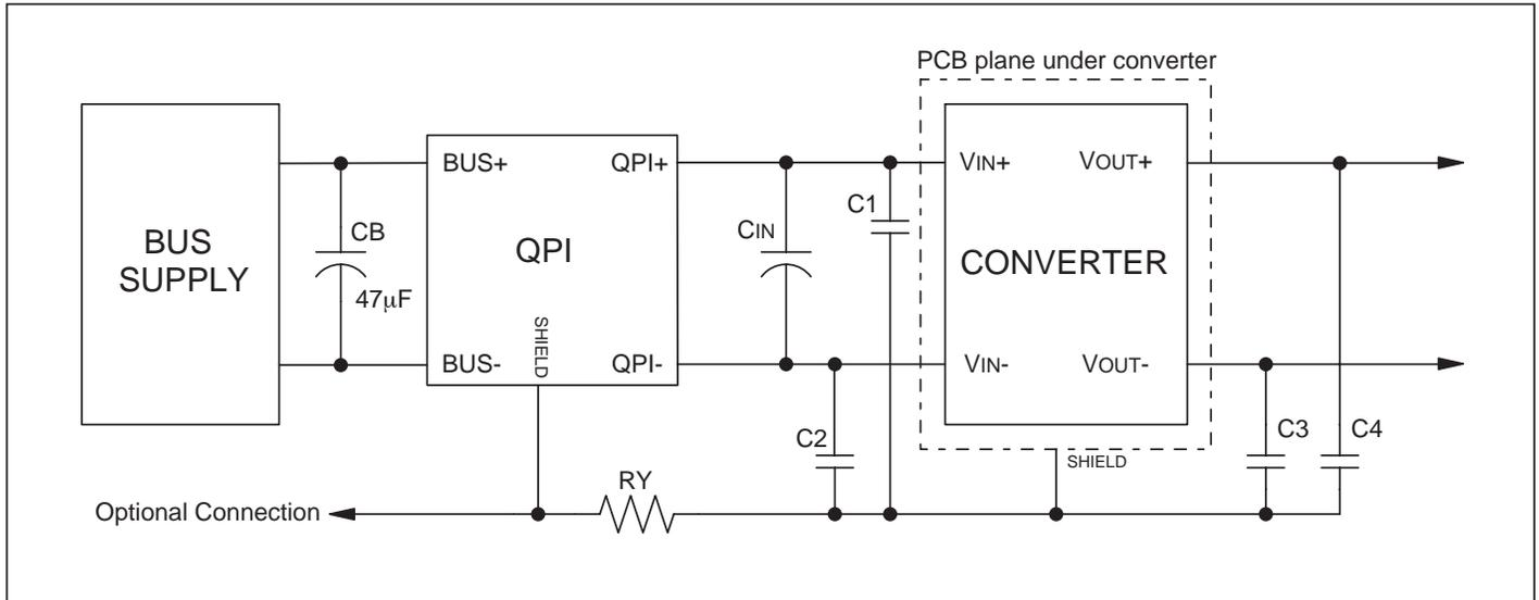
*Figure 6 – Recommended schematic for QPI. Values of C<sub>IN</sub> and C1-C4 should be the values recommended by the converter manufacturer. If the manufacturer does not specify a value for the Y-capacitors use 4.7nF. R<sub>y</sub>=10 Ω, 1/4 W.*
