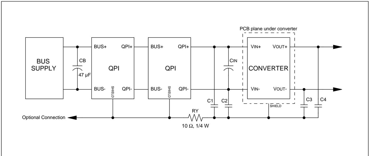
**Figure 8** – Series connection of QPI for higher attenuation.
