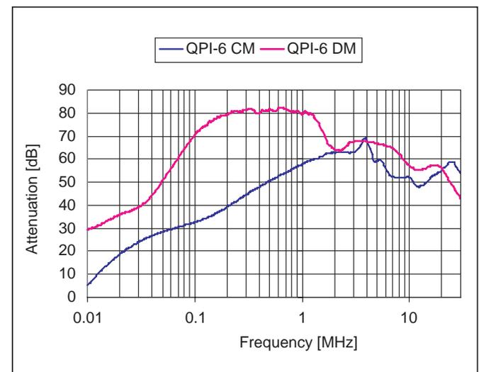
**Figure 2 - Attenuation curves showing common-mode and differential-mode attenuation.**
