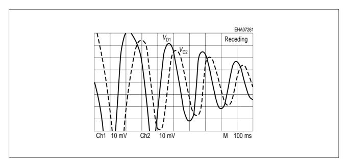
The phase difference between  $V_{\rm D2}$  and  $V_{\rm D1}$  is negative, if the target is approaching the detector.
