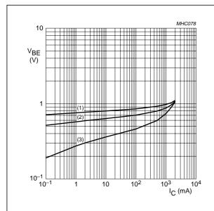
NPN transistor;  $V_{CE} = 5 V$ .
