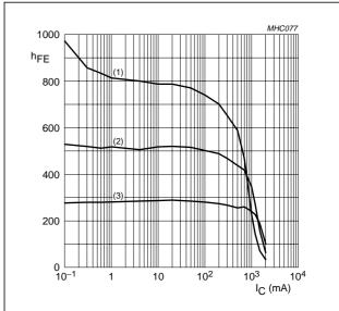
**NPN** transistor;  $V_{CE} = 5 \text{ V}$ .
