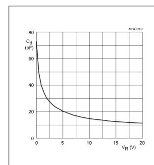
Schottky barrier diode; f = 1 MHz;  $T_{amb}$  = 25 °C.
