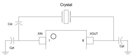
**CST** - Series Capacitor, used to lower circuit load to match crystal load. Raises frequency offset. This can be eliminated by using a crystal with a Cload of equal or greater value than the oscillator.
