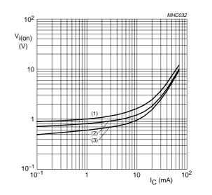
TR1 (NPN);  $V_{CE} = 0.3 \text{ V}.$
