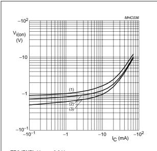
TR2 (PNP);  $V_{CE} = -0.3 \text{ V}.$
