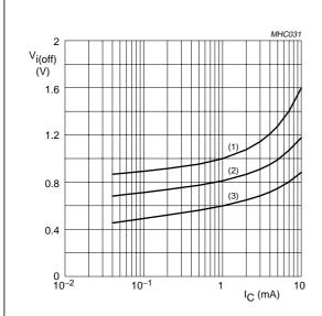
TR1 (NPN);  $V_{CE} = 5 \text{ V}.$
