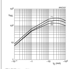
TR2 (PNP);  $V_{CE} = -5 \text{ V}.$
