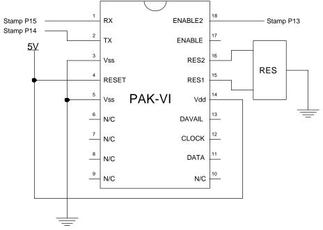
an indication of when the PAK has data available, you can monitor the DAVAIL pin which is high when data is available.
