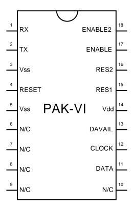
**WARNING:** The PAK VI is a static-sensitive, CMOS device. Observe static precautions when handling. Operating the device without both Vss pins grounded or with RES1 or RES2 disconnected may damage the chip.
