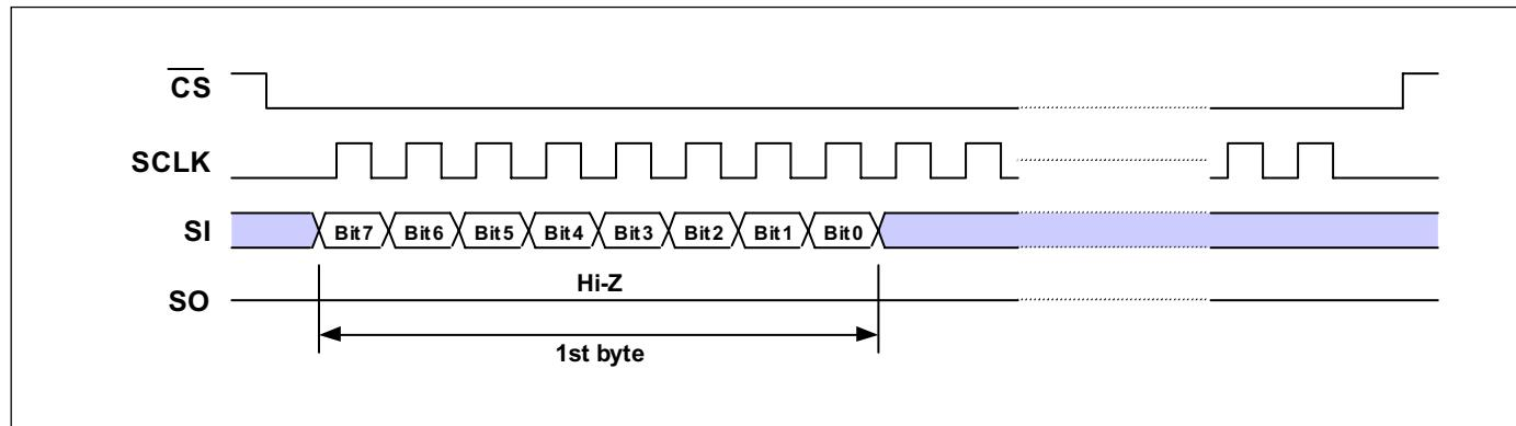
When incorrect command is inputted to this LSI, this LSI becomes standby mode and keeps the standby mode until next CS falling edge. In standby mode, SO pin of this LSI should be High-Z. While  $\overline{CS} = \text{VIH}$ , current=standby current, while  $\overline{CS} = \text{VIL}$  and commands are issuing, or commands are invalid, current=5mA(typ.) to 15mA(max.).
