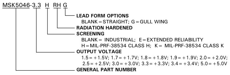
The above example is a +3.3V, Class H screened regulator with gull wing leads.
