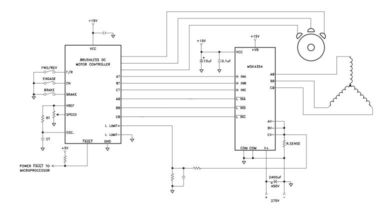
The MSK 4354 is designed to be used with a +270 volt high voltage bus, +15 volt low power bus and +5 volt logic signals. Proper derating should be applied when designing the MSK 4354 into a system. High frequency layout techniques with ground planes on a printed circuit board is the only method that should be used for circuit construction. This will prevent pulse jitter caused by excessive noise pickup on the current sense signal or the error amp signal.
