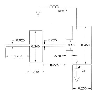
All dimensions are in inches. Substrate material: .025 thick Al<sub>2</sub>O<sub>3</sub>
