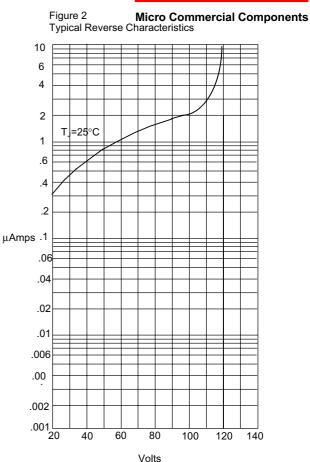
Instantaneous Reverse Leakage Current - MicroAmperesersus Percent Of Rated Peak Reverse Voltage - Volts
