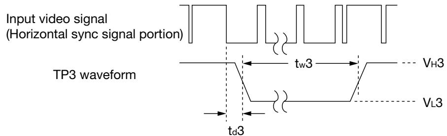
\*7 V. SYNC switching voltage measurement
