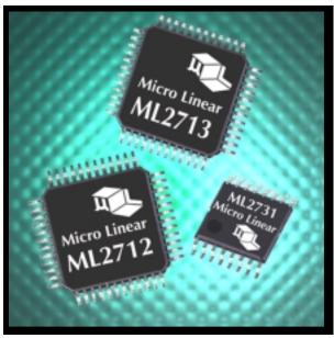
ML2712 2.4GHz Radio Transceiver
