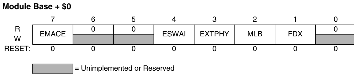
Figure 11-2. Network Control (NETCTL)
