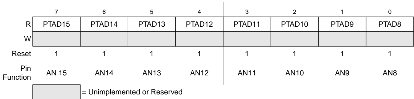
Figure 7-16. Port Data Register 0 (PORTAD0)
