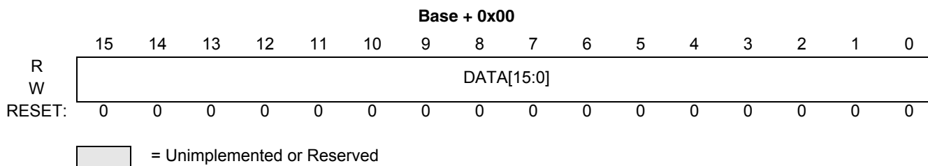
Figure 51. STX Register Diagram
