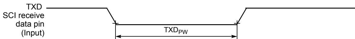
Figure 10-17 TXD Pulse Width
