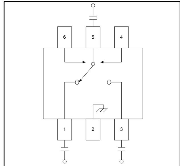
2. DC blocking capacitors are not required if negative control voltage is used.
