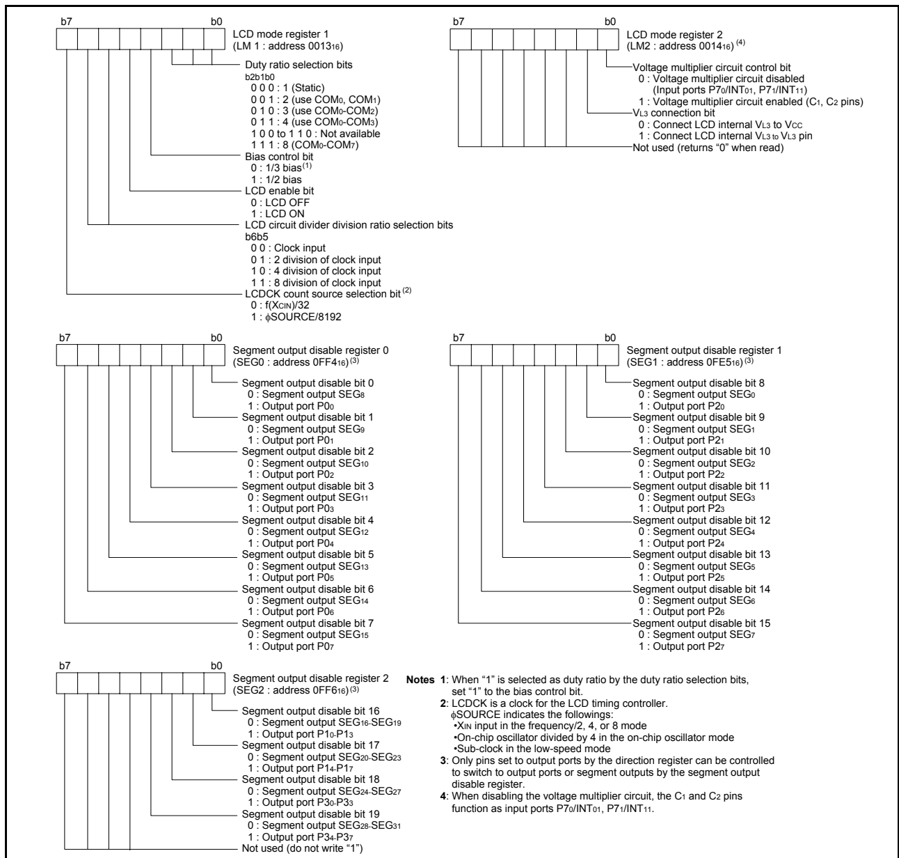
Fig. 43 Structure of LCD related registers
