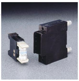
Littelfuse's compact LTFD 101 fuseholders for TLS fuses are designed for quick installation into telecom equipment panels. Their modular design fits into spaces originally designed for circuit breakers and they can be front panel mounted or rear mounted using bullet connectors. The innovative new pull-out design eliminates the need for tools to replace fuses and includes an alarm signaling circuit to identify the blown fuse.
