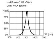
FIG.4 RELATIVE LUMINOUS FLUX VS. WAVELENGTH.
