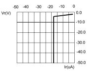
FIG.2 REVERSE CURRENT VS. REVERSE VOLTAGE.
