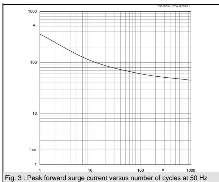
Fig. 3 : Peak forward surge current versus number of cycles at 50 Hz
