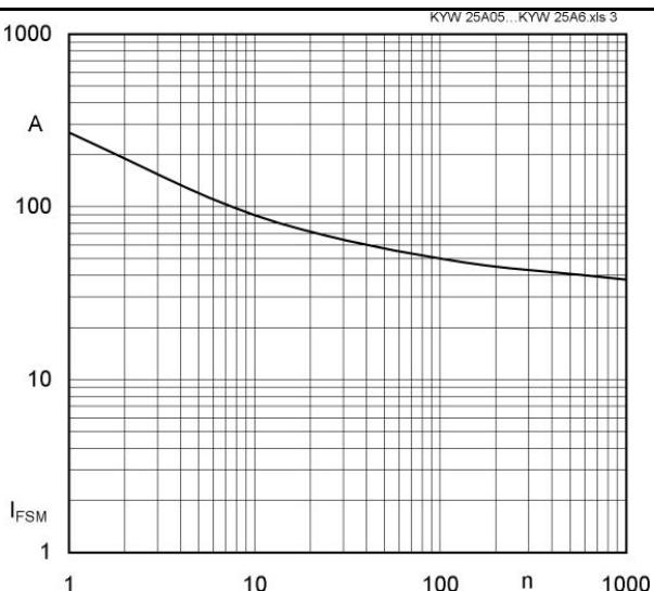
Fig. 3 : Peak forward surge current versus number of cycles at 50 Hz
