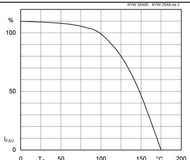
Fig. 2 : Rated forward current vs. case temperature
