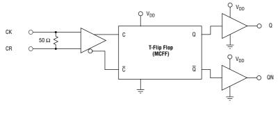
CK CR Q, QN VDD Clock Input Terminal Reference Voltage Bias Terminal Complimentary Data Outputs Power Supply of Internal Circuit
