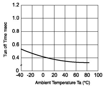
**Fig.5** LED operate vs. ambient temperature
