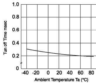
**Fig.5** LED operate vs. ambient temperature
