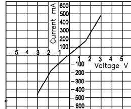
**Fig.9** Off state leakage current
