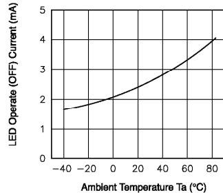
**Fig.6** LED Reverse (ON) current vs. ambient temperature
