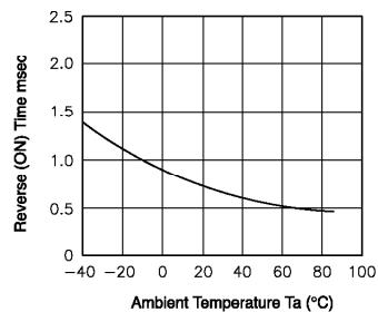
**Fig.5** LED operate (OFF) vs. ambient temperature
