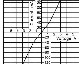
**Fig.9** Off state leakage current
