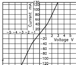
**Fig.9** Off state leakage current
