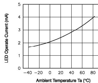
**Fig.6** LED Turn (OFF) current. ambient temperature
