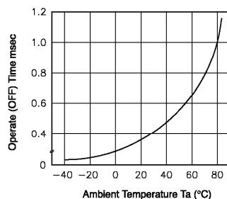
**Fig.4** Turn (ON) time vs. ambient temperature
