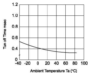
**Fig.5** LED operate vs. ambient temperature
