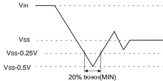
**Note:** For power-up,  $V_{IH} \leq V_{DDQ}+0.3V$  and  $V_{DD} \leq 1.7V$  and  $V_{DDQ} \leq 1.4V$   $t \leq 200ms$
