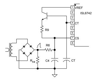
FIGURE 14. ADDING SLOPE COMPENSATION
