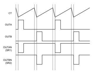
FIGURE 11. BASIC WAVEFORM TIMING
