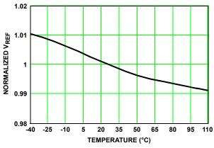
FIGURE 1. REFERENCE VOLTAGE vs TEMPERATURE
