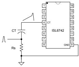
FIGURE 10. SYNCHRONIZATION TO AN EXTERNAL CLOCK
