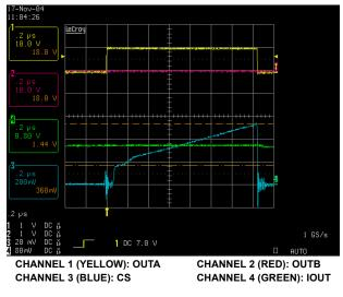
FIGURE 5. CS INPUT vs IOUT
