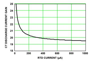
FIGURE 2. CT DISCHARGE CURRENT GAIN vs RTD CURRENT
