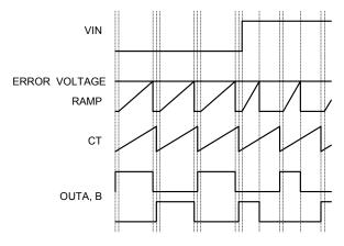
FIGURE 8. VOLTAGE FEED FORWARD BEHAVIOR
