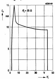
Output Current *I*<sub>o</sub> versus Input Voltage *V*<sub>i</sub>
