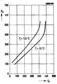
**Delay Switching Threshold**  $V_{\rm dT}$  versus **Temperature**  $T_{\rm J}$
