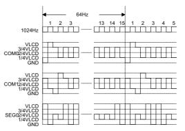
VLCD is fixed at 4.4V when  $V_{DD}$  is from 2.4V to 3.6V.
