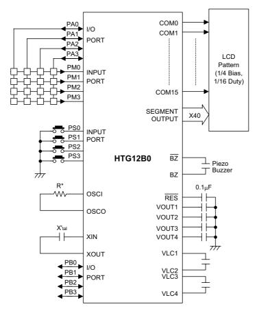
$R^*:$  Depends on the required system clock frequency. (R=620k $\Omega$ ~51k $\Omega$ , at VDD=3V) X'tal: Realtime clock frequency. (X'tal=32768Hz)
