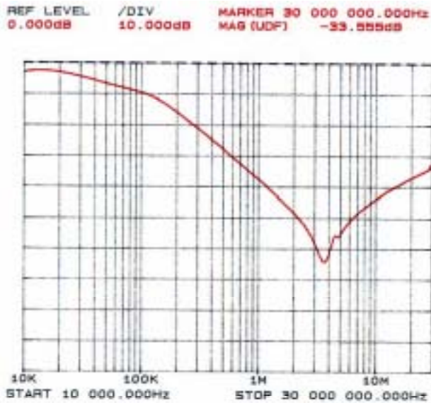
Figure 1: Typical common-mode insertion loss in a 50 circuit
