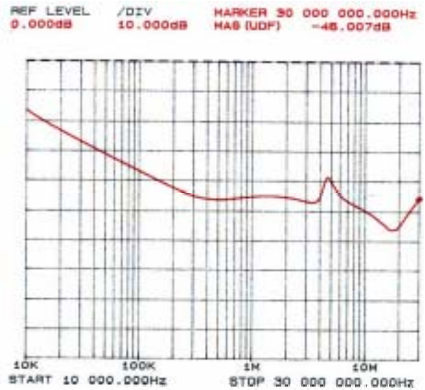
Figure 2: Typical differential-mode insertion loss in a 50 circuit
