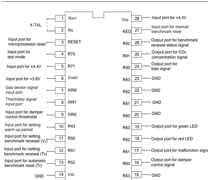
Figure 1 - Pin arrangement for FIC03272
