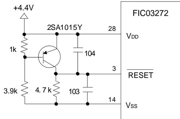
Figure 6 - Reset circuit
