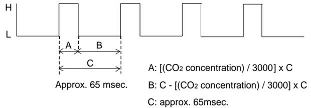
Figure 2 - PWM signal for CO<sub>2</sub> concentration continuously from R63 during this period.
