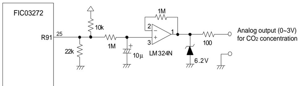
Figure 7 - CO<sub>2</sub> concentration signal circuit
