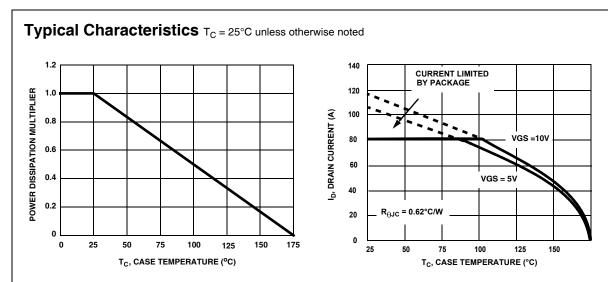
Figure 1. Normalized Power Dissipation vs Case Temperature
