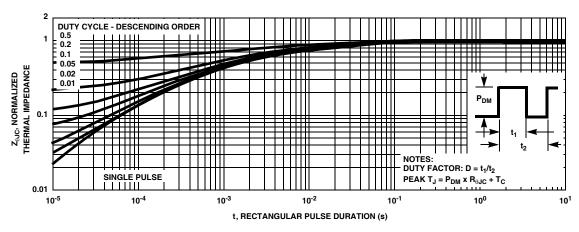
Figure 3. Normalized Maximum Transient Thermal Impedance
