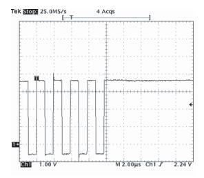
Figure 2: Typical EN/SET Signal.
