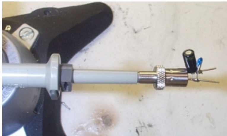
Figure 25 - Oscilloscope Probe with Probe Master 5125BA BNC Adapter. (Modified with wires for probe ground for ripple measurement, and two parallel decoupling capacitors added)
