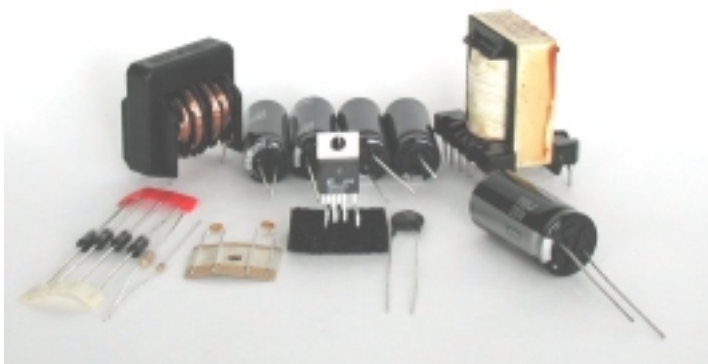
Figure 2 - EP13 230 VAC Input to 115 VAC Input Retrofit Kit.
