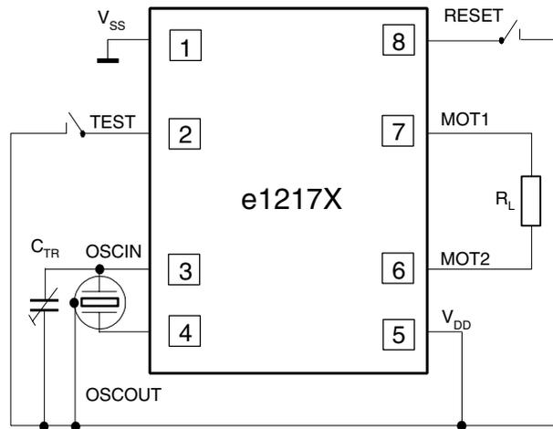
Range of trimmer capacitance:  $C_{TR} = 5 \text{ pF to } 30 \text{ pF}$
