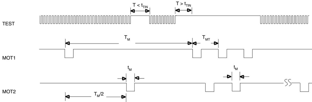
**Figure 4. Motor Drive Outputs and RESET**
