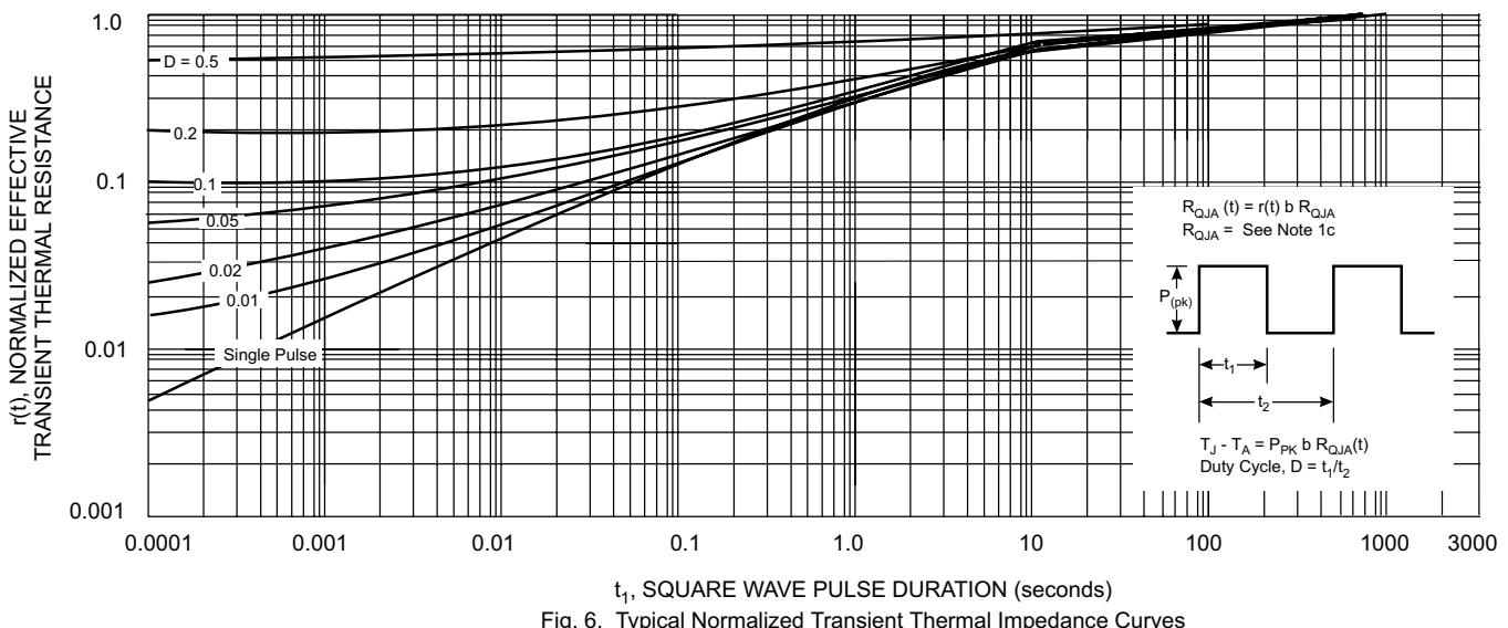
Remark: Thermal characterization performed under conditions described in note 1c. Transient thermal response will change depending on the circuit board design.
