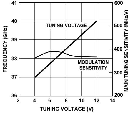
Figure 2. Tuning Voltage vs. Frequency and Modulation Sensitivity.
