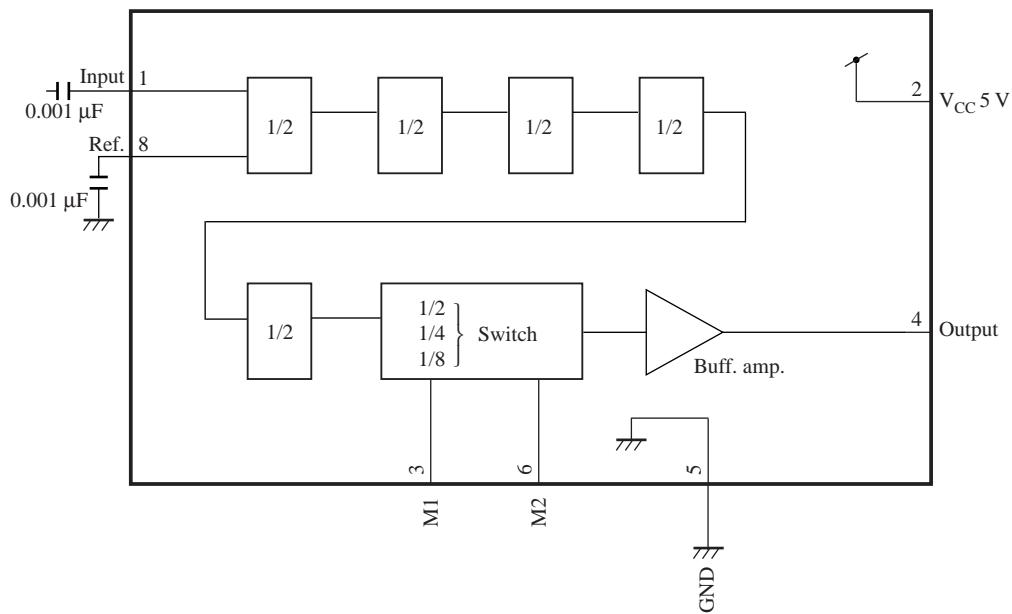
Dividing ratio select pin: M1/M2 settings and related dividing ratios are as follows: High = V<sub>CC</sub>, Low = GND
