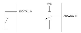
Some of the pins of the DMX710 can be used as digital or analog inputs. In the digital mode you have to connect a switch to GND. The analoge mode permit a signal from GND to VCC.
