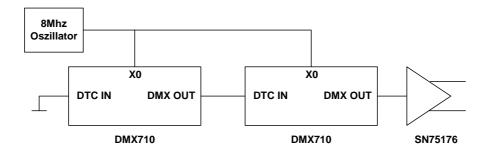
The DMX710 is cascadeable, as the DMX exit is connected with the DTC entrance of the next component. The last DMX exit goes to a line driver. It is possible to use one oszillator for all DMX710.
