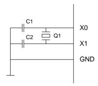
This example illustrates how to use the DMX710 with a 8MHz crystal. The value of the capacitors should be in the range of 12-33pF.
