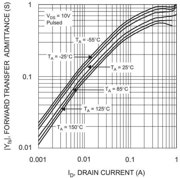
Fig. 10 Forward Transfer Admittance vs. Drain Current
