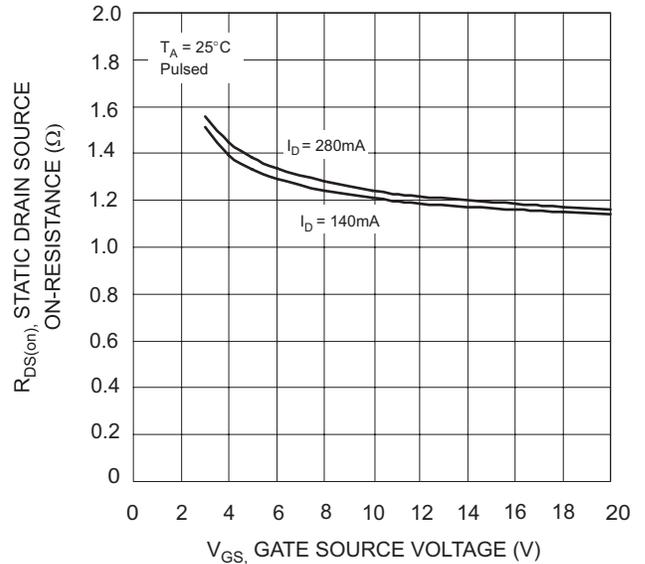
Fig. 6 Static Drain-Source On-Resistance vs. Gate-Source Voltage
