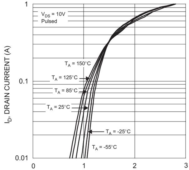
$V_{GS}$ , GATE-SOURCE VOLTAGE (V)
