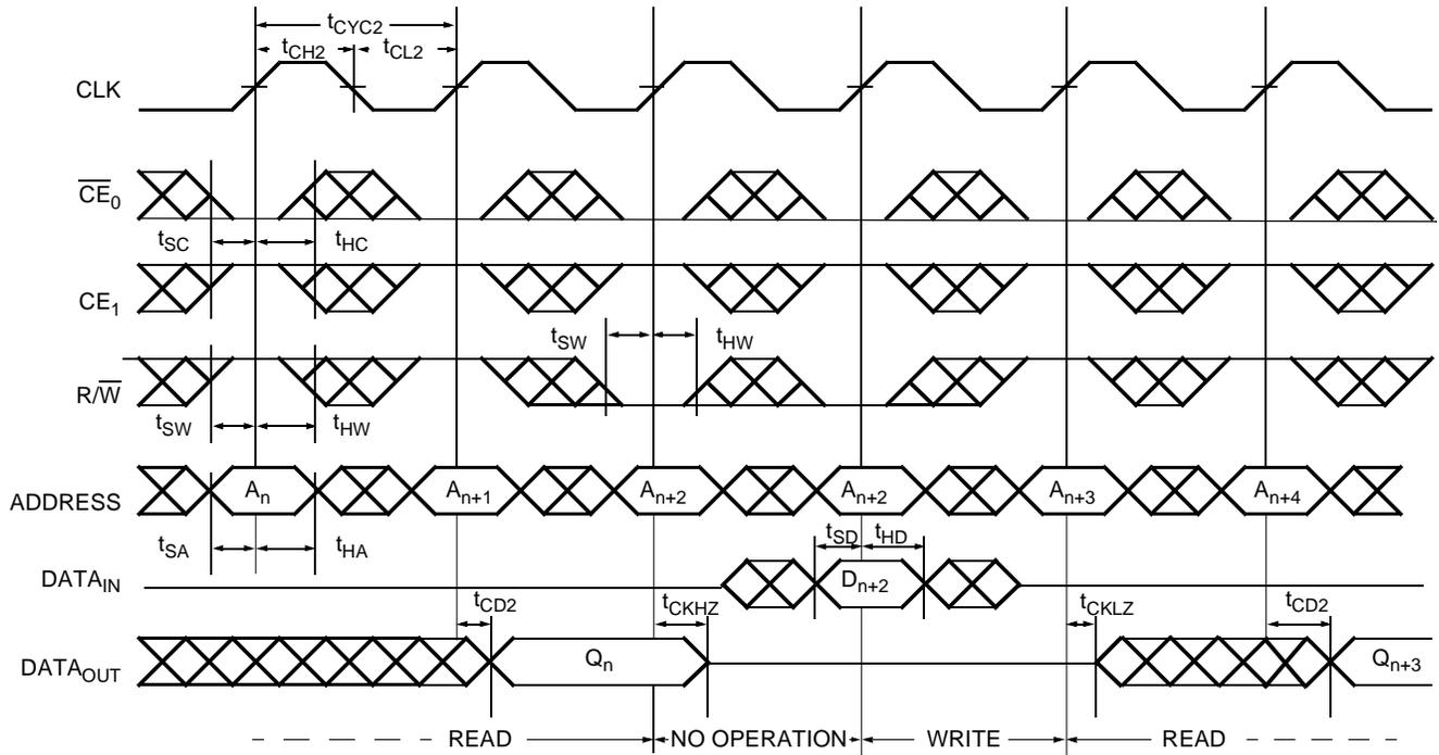
**Pipelined Read-to-Write-to-Read (OE Controlled)** [14, 21, 22, 23]
