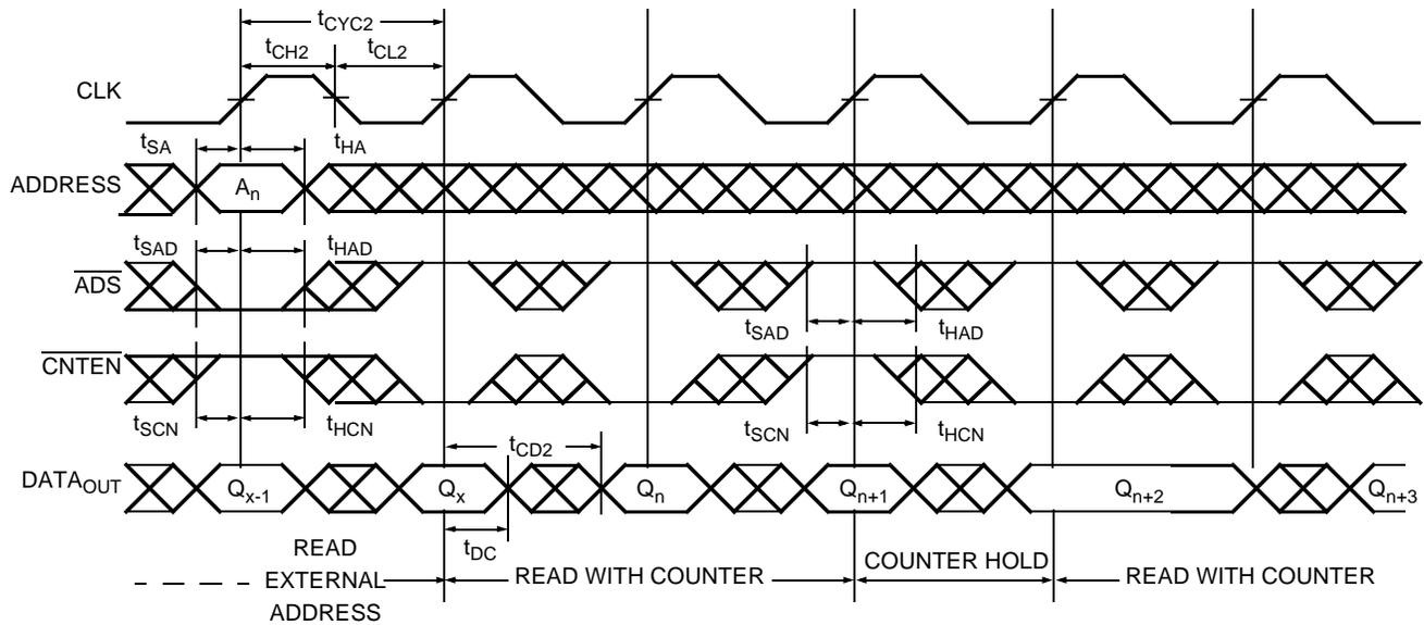
**Flow-Through Read with Address Counter Advance<sup>[24]</sup>**
