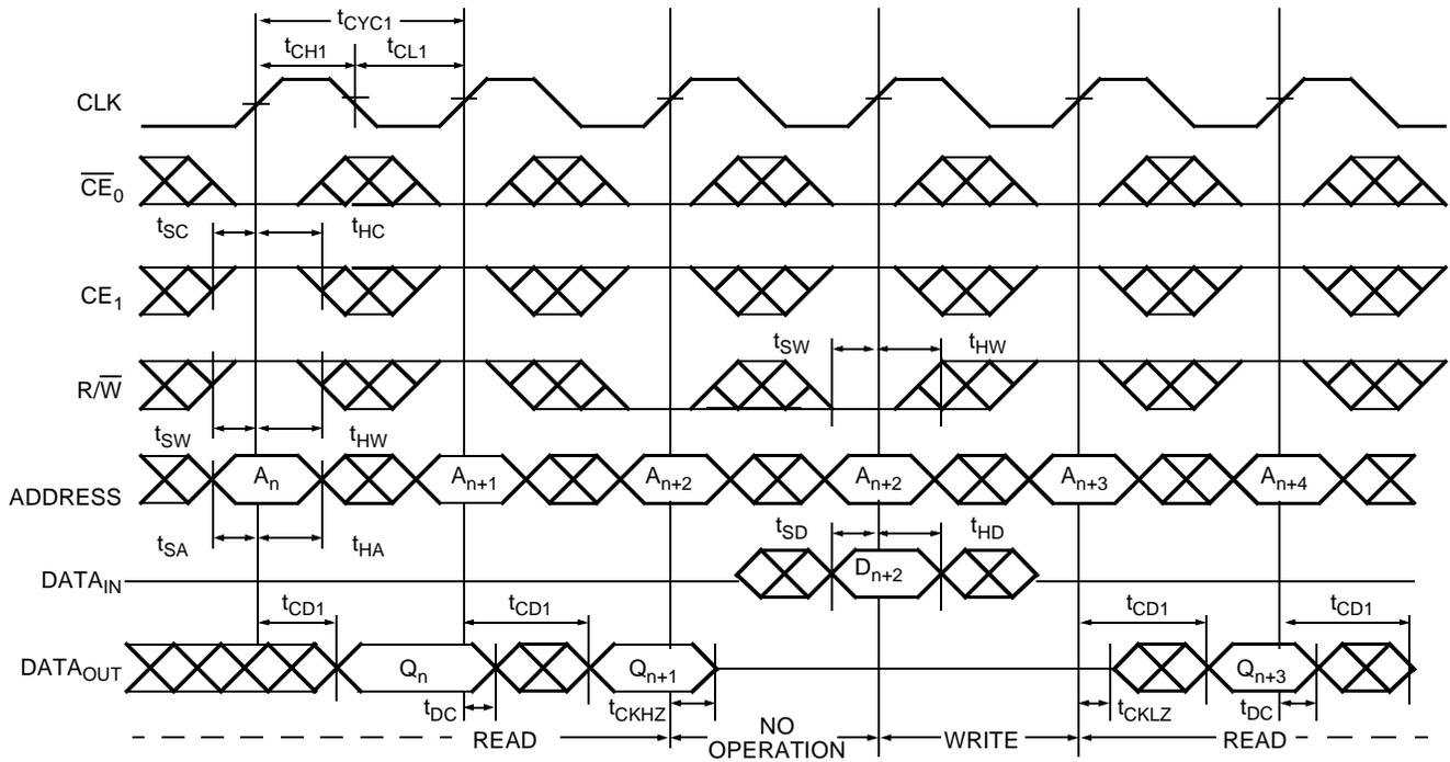
**Flow-Through Read-to-Write-to-Read (OE Controlled)**<sup>[12, 14, 21, 22]</sup>
