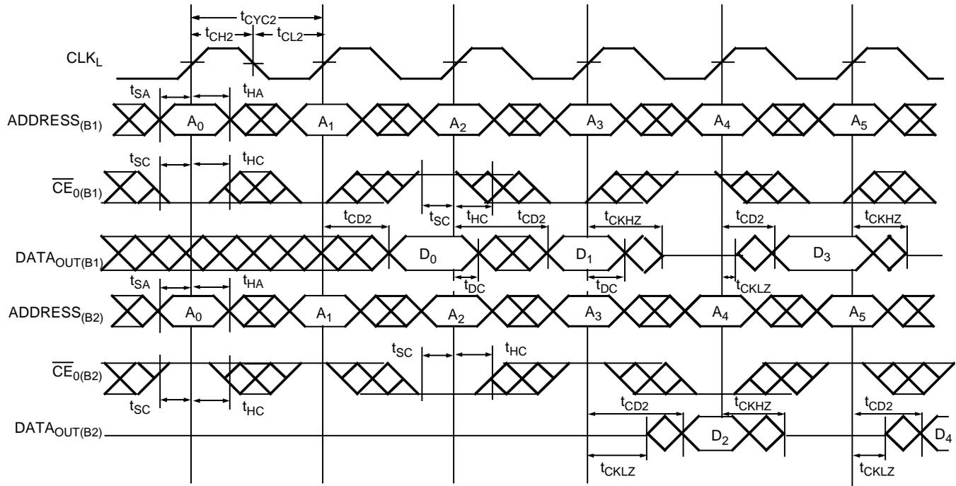
**Left Port Write to Flow-Through Right Port Read<sup>[17, 18, 19, 20]</sup>**
