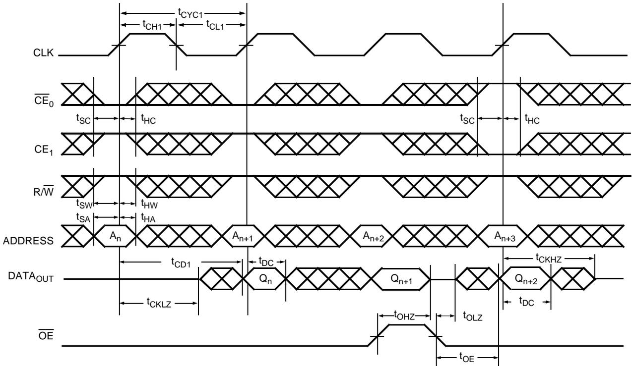
Read Cycle for Pipelined Operation ( $\overline{FT}/PIPE = V_{IH}$ )<sup>[11, 12, 13, 14]</sup>
