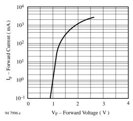
Figure 3. Forward Current vs. Forward Voltage
