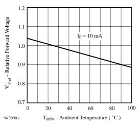
Figure 4. Relative Forward Voltage vs. Ambient Temperature
