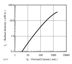
Figure 5. Radiant Intensity vs. Forward Current
