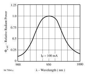
Figure 8. Relative Radiant Power vs. Wavelength
