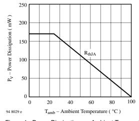
Figure 1. Power Dissipation vs. Ambient Temperature
