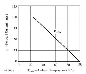
Figure 2. Forward Current vs. Ambient Temperature
