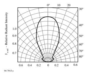
Figure 9. Relative Radiant Intensity vs. Angular Displacement
