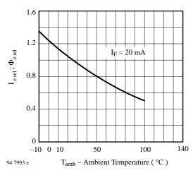
Figure 7. Rel. Radiant Intensity\Power vs. Ambient Temperature
