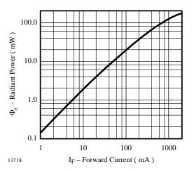
Figure 6. Radiant Power vs. Forward Current
