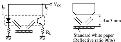
\*2 Time required for the collector current to increase from 10% to 90% of its final value.
