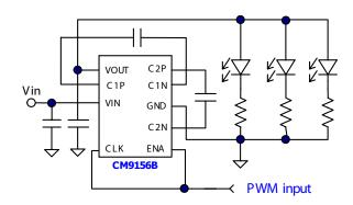
Figure 3. PWM brightness control, lowered quiescent current
