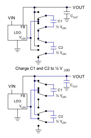
Figure 1. Switch operation
