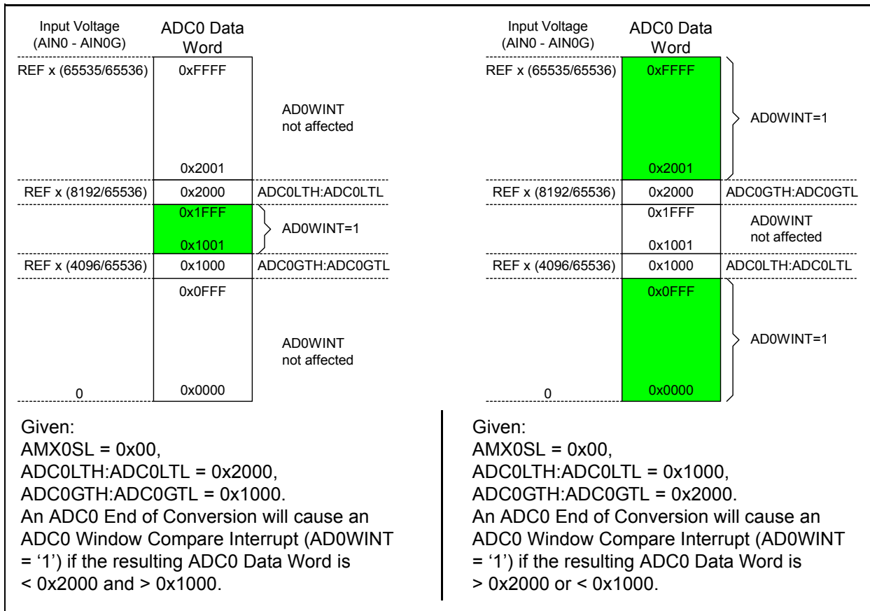
Figure 5.28. 16-Bit ADC0 Window Interrupt Example: Single-Ended Data
